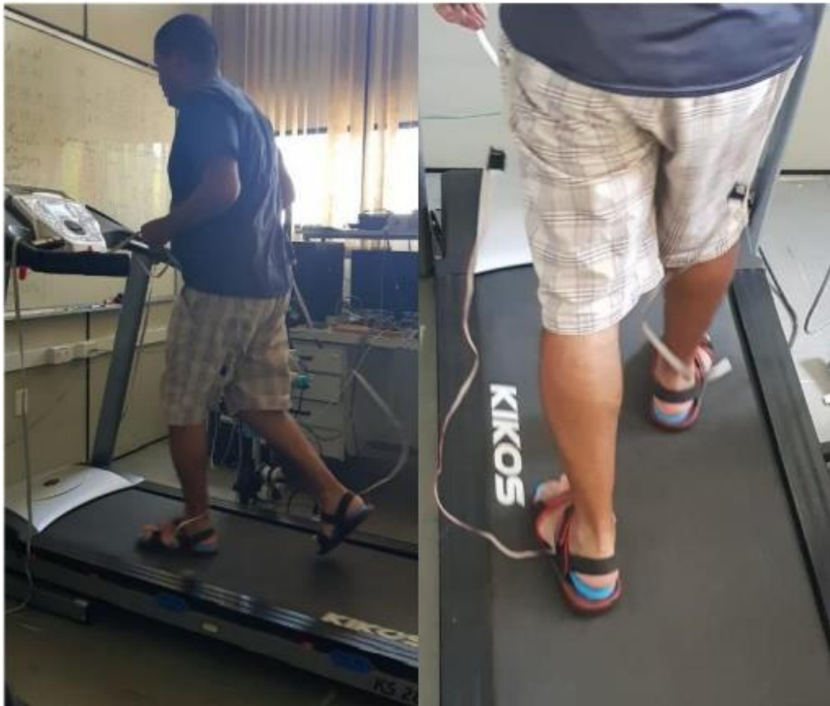
Fig. 7. Tests carried-out with the National Instruments module: (on left) View of the test condition and (on right) view of the test in detail of the feet with the proposed insole on the right foot. The insole in the left foot is outside of the focus of this paper and was fabricated using piezoelectrets sensors.
