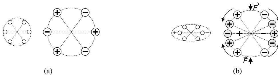
Fig. 1. Example of crystalline structure of a piezoelectric material: (a) before application of a force; (b) after application of a force [7].
